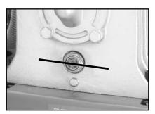
Figure 3. Proper oil level.
